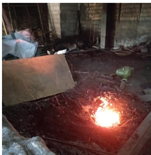
Figure 1. The process of smelting tin and copper to produce bronze as raw material for gamelan
