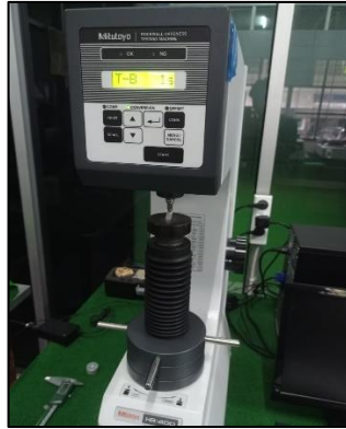
Gambar 6. Mesin Hardness Tester Mitutoyo HR-400
