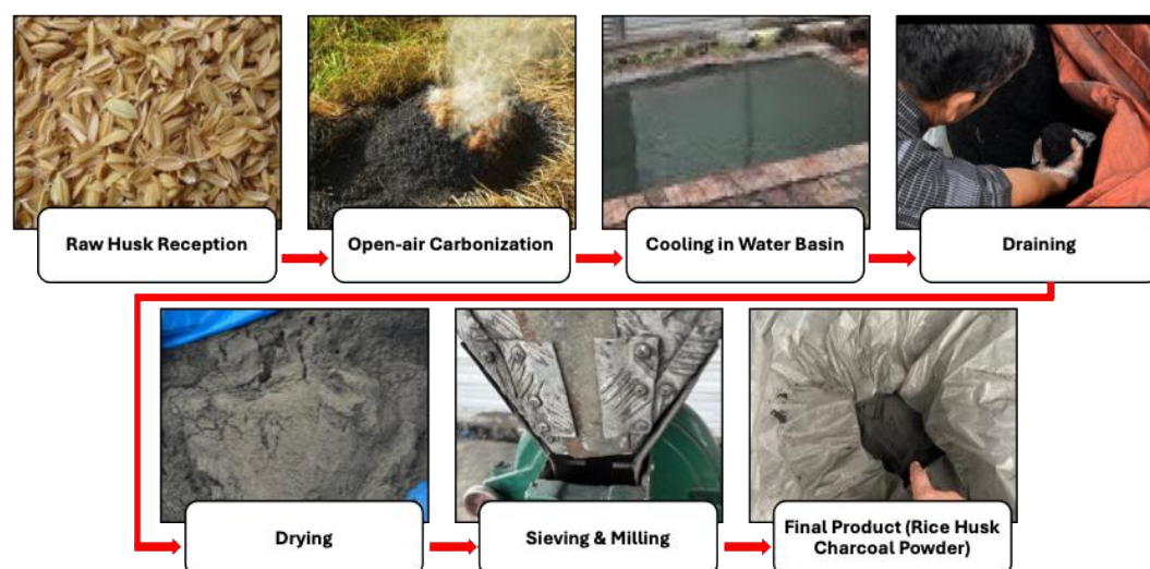
Figure 1. Production process mapping of rice husk charcoal powder
