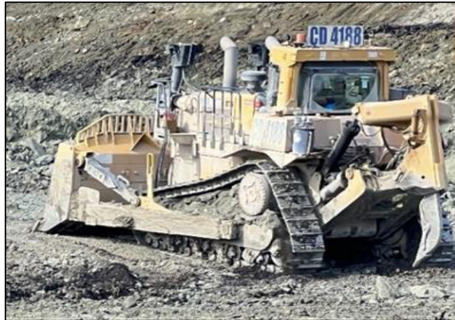
Gambar 5. Bulldozer Ripper Caterpillar D10R
