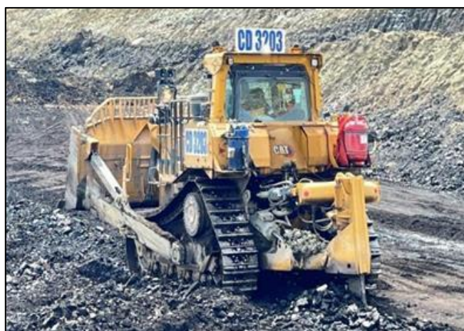
Gambar 6. Bulldozer Ripper Caterpillar D10R
