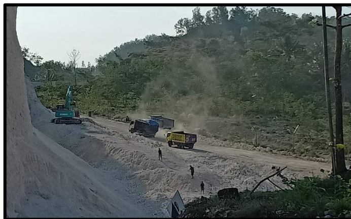
Gambar 3. Kondisi Tidak Aman Akibat Jalanan Berdebu Fig 3. Unsafe Condition Caused by Dusty Track
