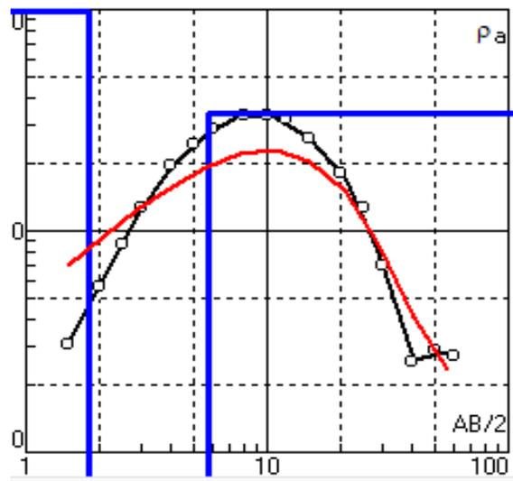
**Fig. 3.** Results of Data Processing Resistivity to Depth on Sounding 2**Table 2.** Data Interpretation.
