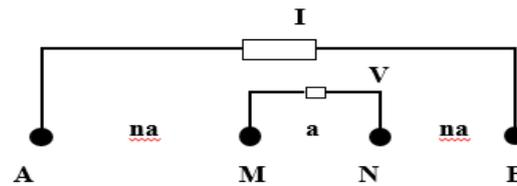
Fig 1. Schlumberger Configuration Electrode Arrangement.
