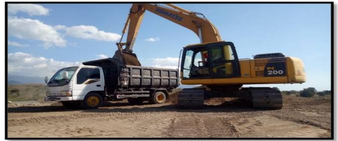
Gambar 1 Alat Gali-Muat Excavator tipe back hoe merk komatsu PC 200 – 3
