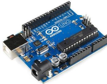
**Gambar 1.** Arduino ATmega 328P
