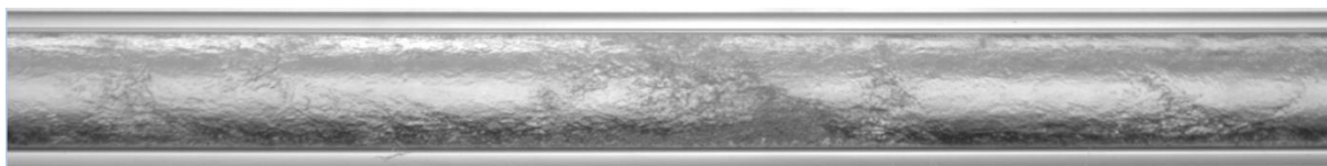
Figure 6. Annular flow ( J_G 14 m/s and J_L 0.2 m/s)
