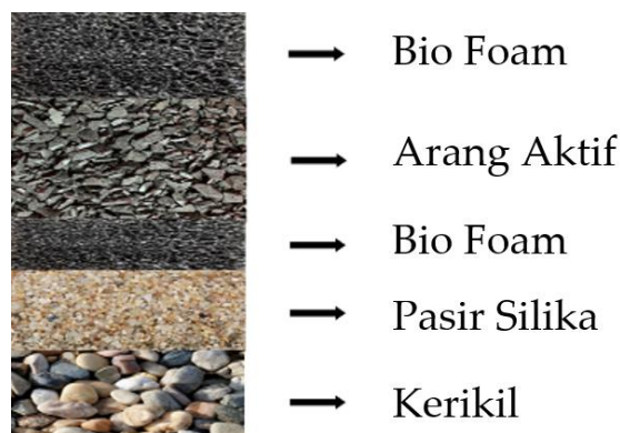
Gambar 2. Susunan Media Filter Air
