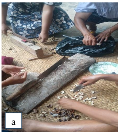
Gambar 4a. Alat kacip manual jambu mete
