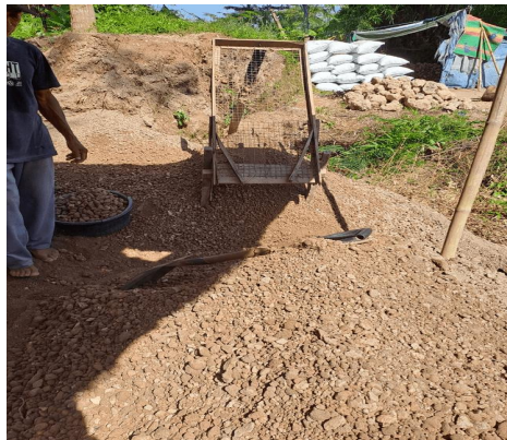
Figure 1. Sieving Process of Pumice as Paving Material
