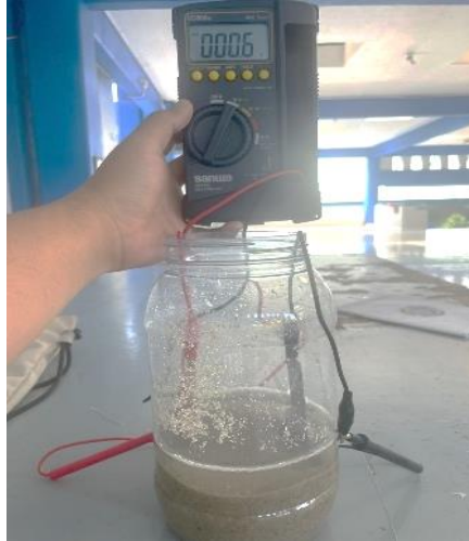
Figure 1. Electrochemical cell circuit using seawater and sea sand
