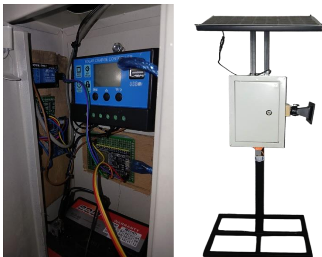
Figure 4. Ultrasonic Pest Repeller Based on ESP32 and IoT
