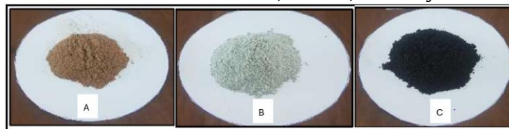
Figure 2. Activated adsorbent material: A)claystone, B)zeolite, C)coconut shell
