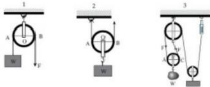
Gambar 3.3. Prinsip Kerja Katrol
