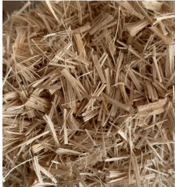
Figure 4. Abaca fibers cut into 5 cm lengths
