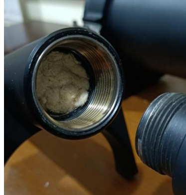
Figure 6. Abaca-wool testing using an impedance tube with a diameter of 3 cm
