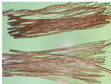
Figure 1. Fibers specimen (a) banana fiber and (b) coconut fiber
