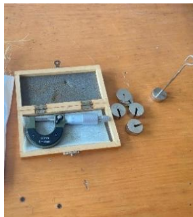
Figure 2. Equipment used: (a) screw micrometer, (b) weights
